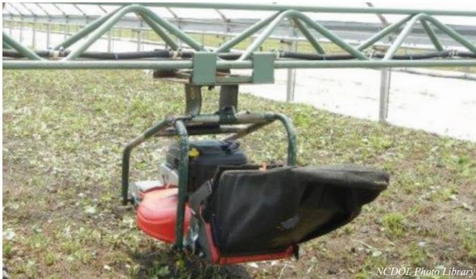
*Modified mower mounted on boom.*
