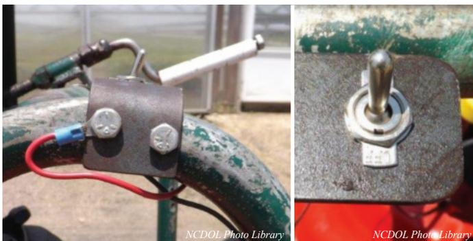
*Toggle switch used to activate modified mower.*
