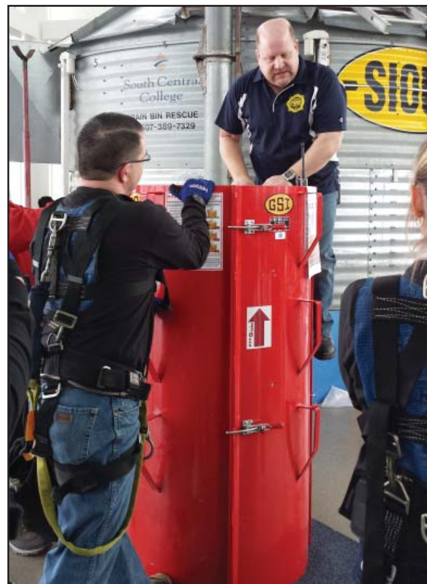
Trained professionals demonstrate how a rescue tube works to free someone from grain.
